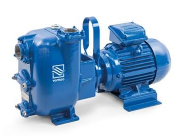
**Product Data** Suction port Threaded - 3" ISO 228 (BSP) Delivery port Threaded - 3" ISO 228 (BSP) Qmax 95 m<sup>3</sup>/h - 1583 l/min (418 USgpm) Hmax 16 m (52 ft) Solids handling 40 mm (1,5 ") Motor power 4 kW - 5,5 HP Motor type **IEC** standard Winding for inverters **Cast iron frame** Motor brand WEG W22 Premium Weight 112 ka
